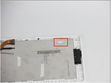
Depress power switch using finger, and simultaneously pry in same direction with a plastic opening tool. To reassemble your device, follow these instructions in reverse order.
