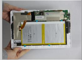
Using the metal spudger, carefully pry open the back cover.
