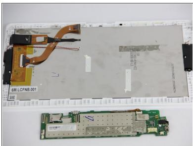
Using the small plastic tool, carefully pry the motherboard out of the device.
