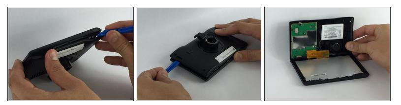
• Using the plastic opening tool, pry apart the device around the seam.
