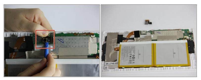
Use the plastic opening tool to pry up the rear facing camera. Once removed the front facing camera will come out as well.
