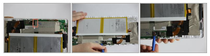
Using the plastic opening tool gently place the tip of it under the connection and pry up. It will pop out.
