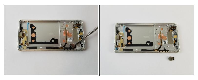
• Remove the vibration motor from the frame.
