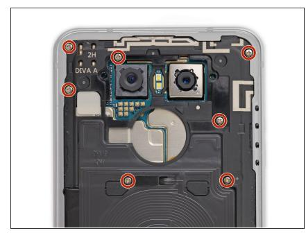
Remove the seven Phillips screws holding down the upper antenna shield.
