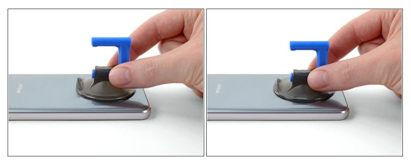
• Secure a suction cup to the rear panel, as close to the heated edge as possible.
