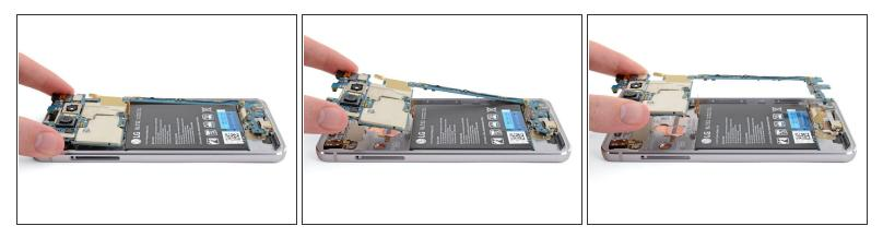
• Grab the motherboard by the top end (the end with the cameras) and gently lift it up and out of the phone.
