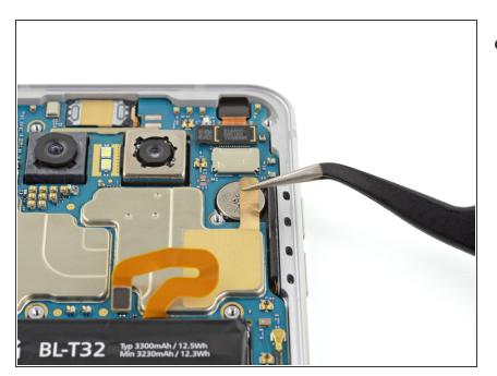
• Remove the sticker connecting the motherboard to the vibration motor.
