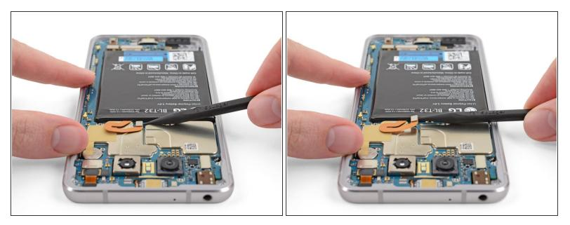
Use a spudger to pry up the press connector at the end of the battery's ribbon cable, disconnecting the battery.
