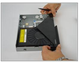
Lightly lift off the hook on both front rear side and the bottom of the device to remove the front panel
