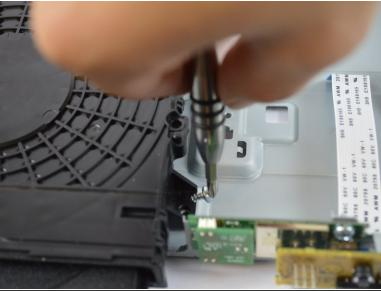
Remove the two screws that attach the disk drive to the frame using a #1 Phillips screwdriver.
