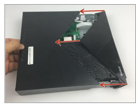
Pull the top cover off by sliding back from the device once the screws have been taken out.
