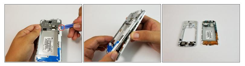
• Use the plastic opening tool to remove the back housing from the frame of the phone.
