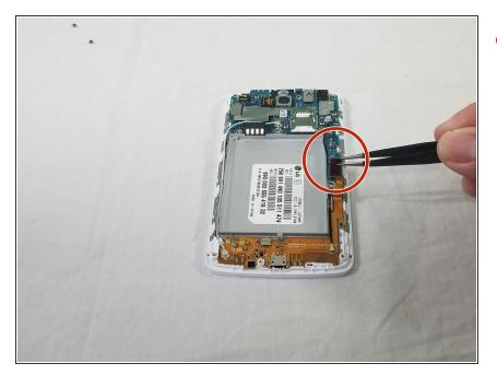
• Lift copper tab located on the right side of the device.
