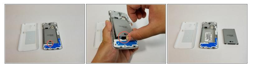
• With your finger, pry the battery out through the crease made for removal.
