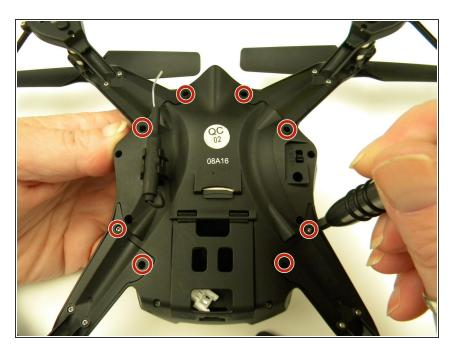
Remove the eight (8) 5mm screws attaching the motor arms to the body using a JIS #00 screwdriver.
