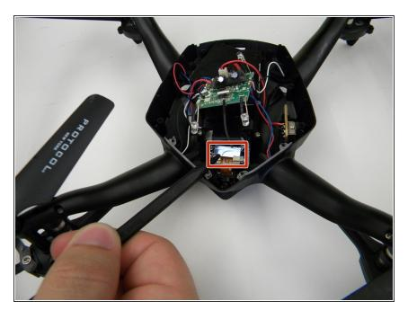
Move the ribbon cable out of the way with the Spuger.
