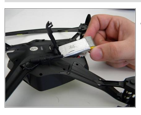
Remove battery pack from body of drone.
