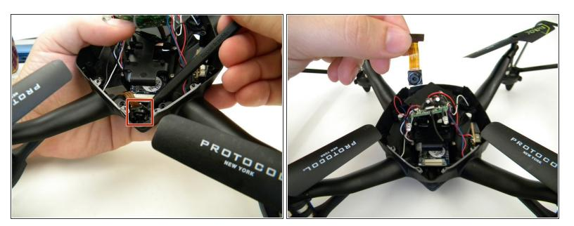
Remove the camera by gently prying it out of the bracket with the spudger.
