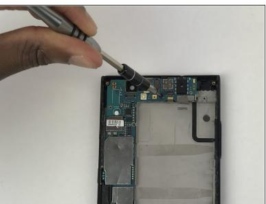
With the same screwdriver, remove the two screws from the motherboard.
