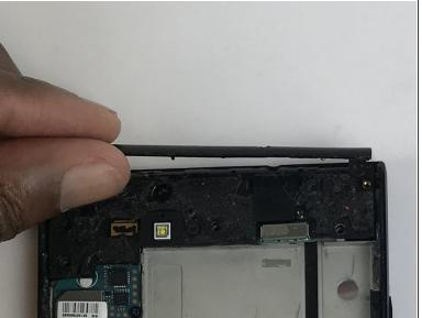
• Use a plastic opening tool to remove the plastic piece in the upper part of the phone.
