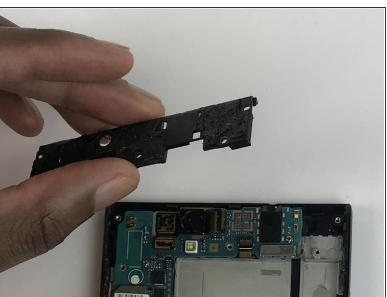
Use the same tool to pry off the plastic that is covering the motherboard.
