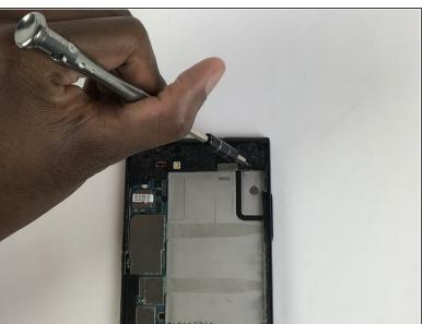
Use a screwdriver with a JIS #000 head to remove the (8) eight screws.
