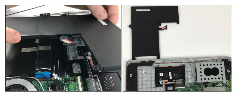
• Remove the battery from the device.
