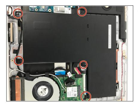
Use the Phillips #0 screwdriver to remove the five 4mm screws around the battery.
