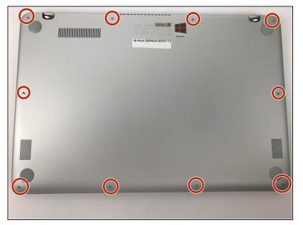
Use the T5 Torx screwdriver to remove the ten 1mm screws located around the back cover.
