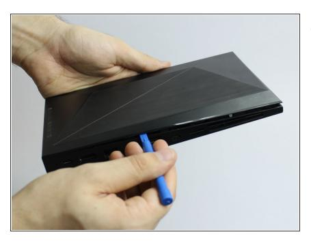
Flip the device over and use a plastic opening tool to remove the bottom cover.
