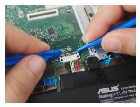
Placing two plastic opening tools on each side of the battery connector and gently pull with an even force on both sides of the connector until the connector pops out.
