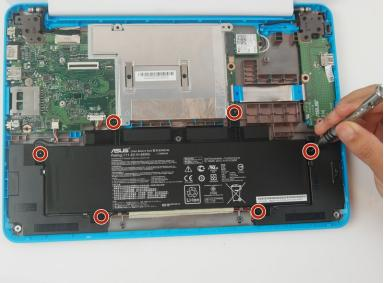
Remove (6) six "4mm" screws that hold the battery using the Phillips #000 screwdriver.
