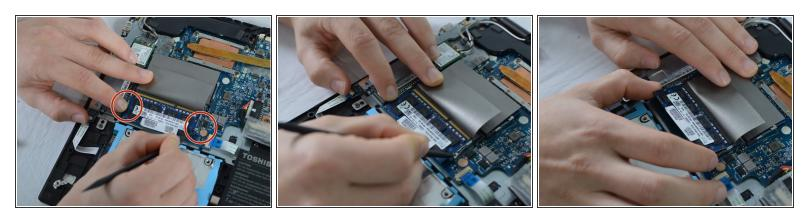
Push outwards on the metal tabs located on both sides of the RAM to release the RAM. You can
