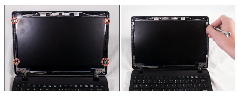
• Using the JIS #1 screwdriver, remove the 4 3mmscrews from each corner of the screen
