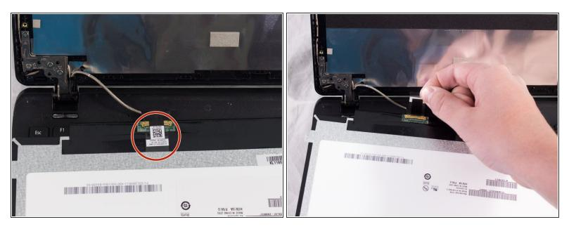
• Carefully pull back the tape on the connector until the connector is fully revealed
