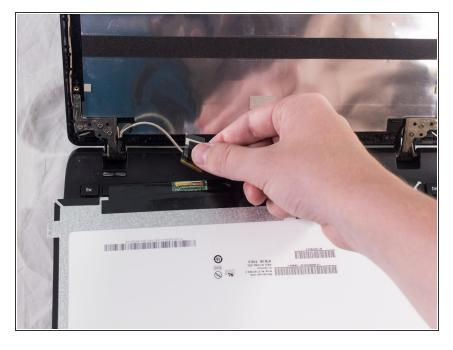
Carefully remove the connector from the old screen and connect it to your new, compatible screen
