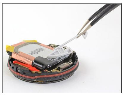
Use <u>tweezers</u> to lift out the grey plastic cover over the battery connector.
