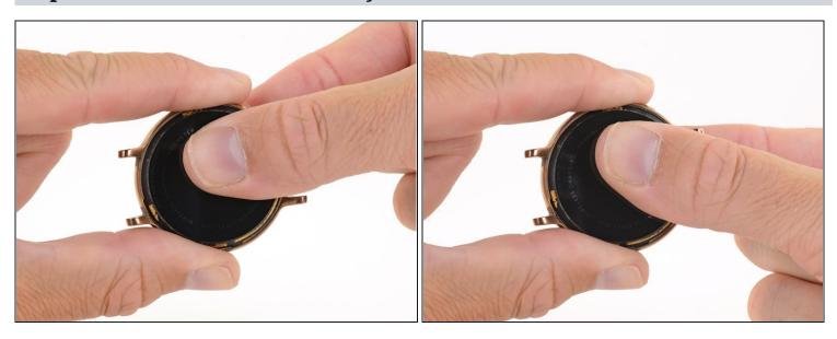
• While holding the outer case steady, twist the inner watch assembly clockwise until it stops.
