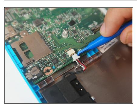
Use a plastic opening tool to remove the connection from sound driver on the bottom left of the motherboard.
