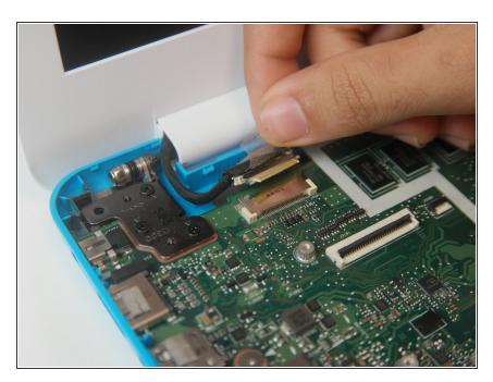
Start by lifting tape up off of the connection. Remove the connection to display.
