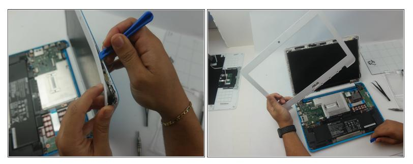
Using the plastic opening tool, separate the display cover bracket from the back of the display.
