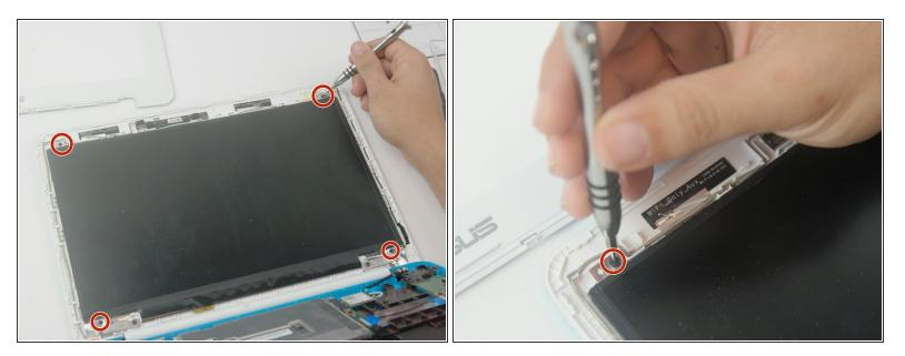
Remove the (4) four "4mm" screws in each corner that hold the display using the Phillips #000 screwdriver.
