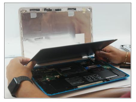
• Lower the display to allow access to connector in back.
