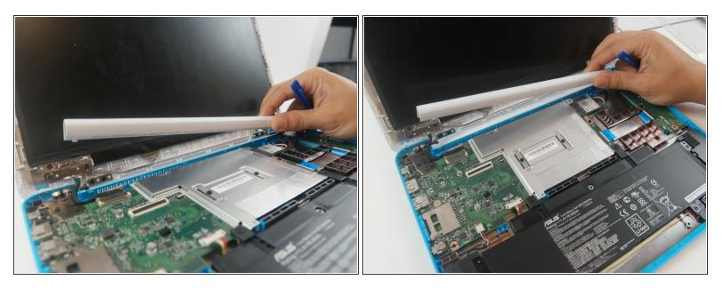
Remove the hinge protector by using the plastic opening tool to gently lift it up. It should come up easily.
