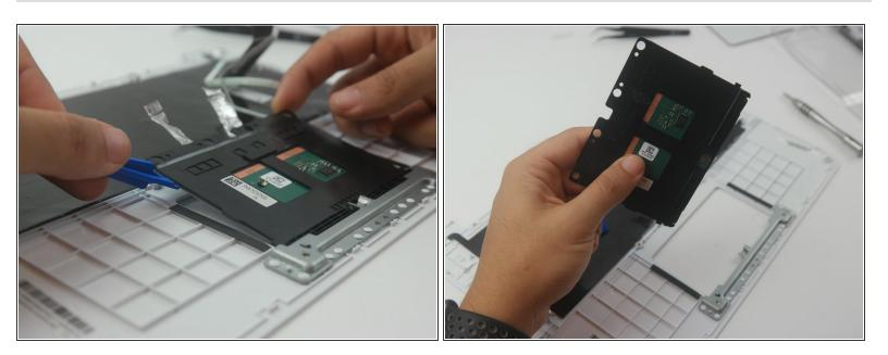
Using a plastic opening tool, pry out the touchpad from the metal securing bracket.
