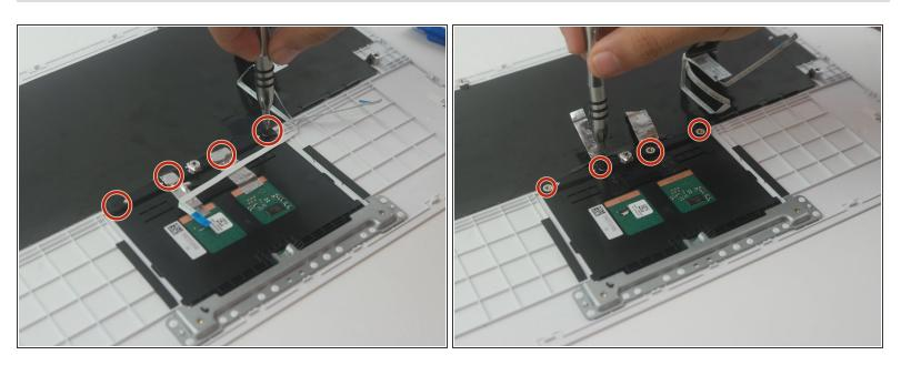
Using the Phillips #000 screwdriver, remove the (4) four "4 mm" screws that secure trackpad onto keyboard.
