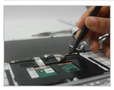
Remove the aluminum tape that secures the trackpad. Use tweezers if necessary.
