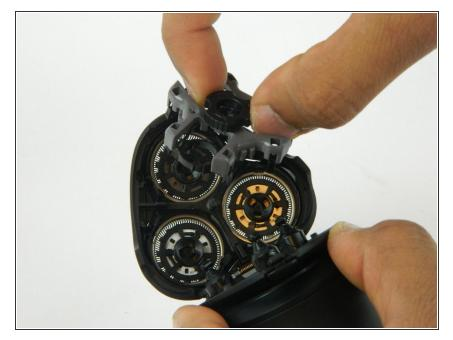
• Remove the head seat from the device.
