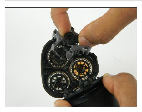
Remove the head seat from the device.
