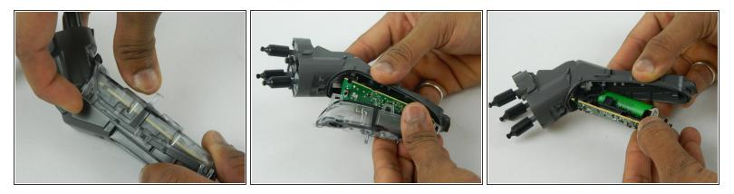
Remove the clear case that holds the circuit board by lifting the latches on the sides and then pulling gently.
