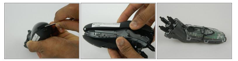
• Pry the remaining casing open using a metal spudger.
