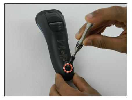
Remove the single screw on the back casing using a T8 Torx screwdriver.
