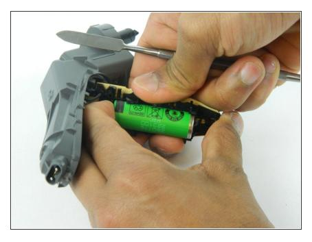
Located directly behind the circuit board, remove the battery from the device.
