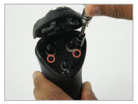
Remove the two 10.1 mm screws inside the shaver head using a T8 Torx screwdriver.
