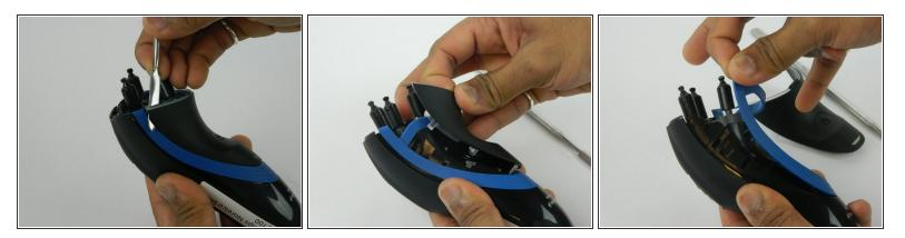
• Gently pull the black and blue casing apart using a metal spudger.
