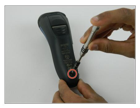
Remove the single screw on the back casing using a T8 Torx screwdriver.
