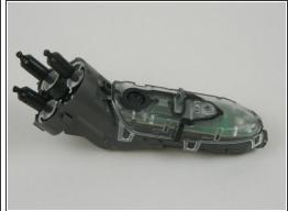
Pry the remaining casing open using a metal spudger.
