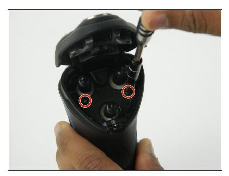
Remove the two 10.1 mm screws inside the shaver head using a T8 Torx screwdriver.
