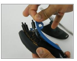
• Gently pull the black and blue casing apart using a metal spudger.
