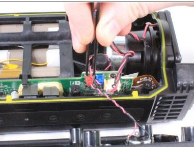
Using a pair of tweezers or your hand, carefully remove the red bundled cable connectors from the motherboard.
