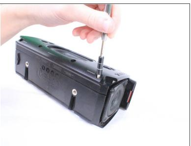
Using a #2.0 Hex screwdriver to unscrew the 8 12mm screws depicted.
