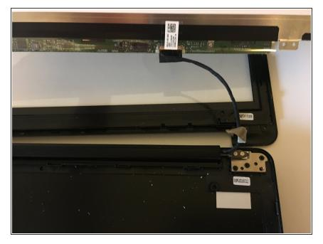
Pull the screen horizontally away to remove the last cable attached to the screen.
