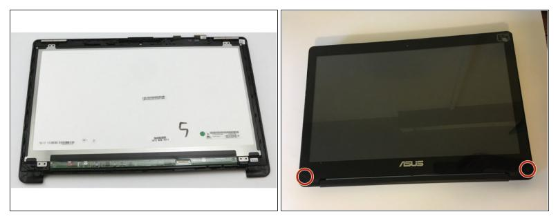
• Remove the two screw covers by hand or by using the pointed end of a spudger.
