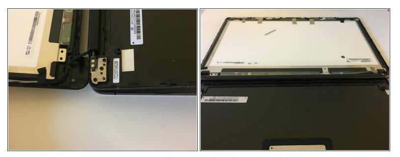
• Separate the two parts of the screen.
