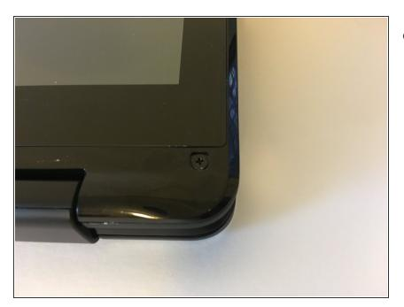
Remove both screws with a Phillips head screwdriver.
