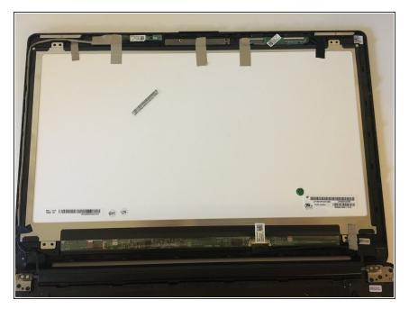
• Remove any tape that is holding the screen in place.
