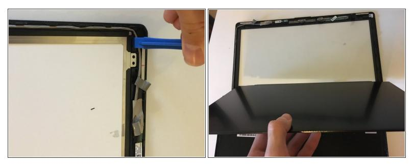
• Use an opening tool to lift out the screen after all the tape is removed.
