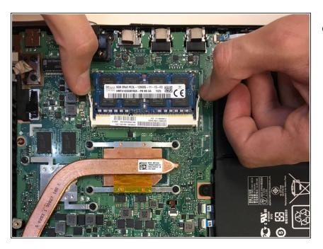
Gently lever the two arms securing the RAM toward either side of the laptop, while holding the RAM in place with your thumbs.
