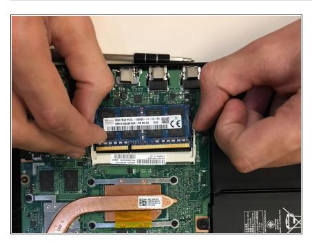
Carefully slide the ram with your index fingers from in between the white tabs.
