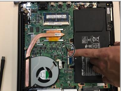
On the bottom of the laptop, gently pull the wire connecting the battery to the motherboard
