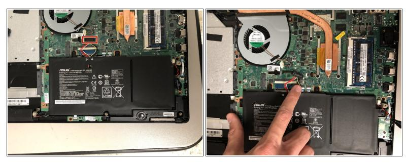
• Disconnect the wires at the top of the battery by lifting on the tabs protruding out of the plastic frame.
