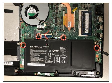
Remove the four screws holding the battery in place, two on top and one on each side.
