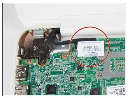
• Unplug the cable located in the upper left corner of the device.
