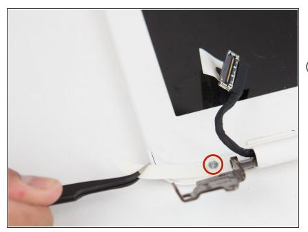
• Remove these tabs located at each of the bottom corners of the display.
