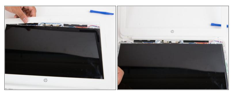
• As you work the plastic opening tool around the edge, remove the front frame of the device.
