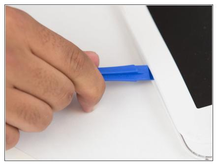
Insert the plastic opening tool and work it around the entire frame of the display.
