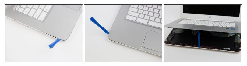
• Open the laptop and place it upright. Remove the keyboard from the device using a plastic spudger or opening tool.
