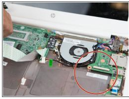
• Carefully remove the (3) three plastic strips attached to the motherboard.
