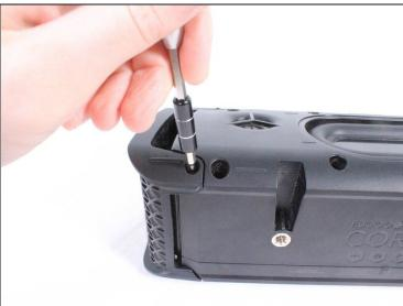
• Remove the 8 screws (4 on each side) that hold the covers that conceal the bass speakers. Remove these 3mm screws using a #2.0 Hex screwdriver.
