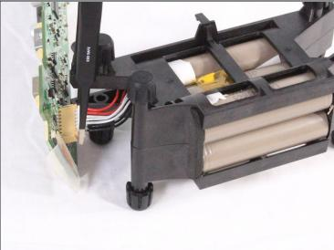
• Using tweezers or your hand, carefully disconnect the bundled cables connecting the battery to the motherboard.
