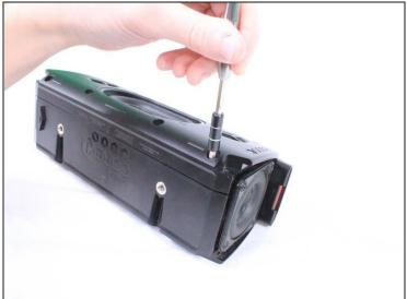
• Use a #2.0 Hex screwdriver to unscrew the 8 screws shown in the image.
