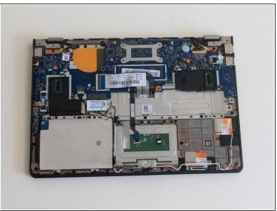
After you have unscrewed the screws, unplugged the cable, and removed the tape and wires, you can remove the battery from your laptop.
