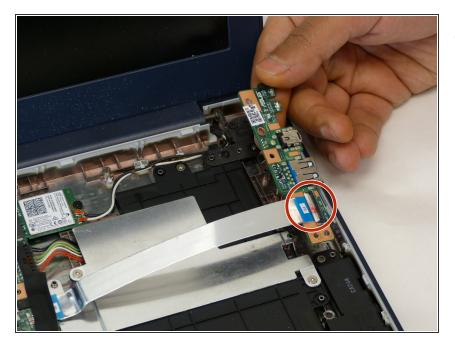
Gently remove the thin band from the daughterboard. You may have to use a thin blade or spudger to lift the silver clip to release the band.
