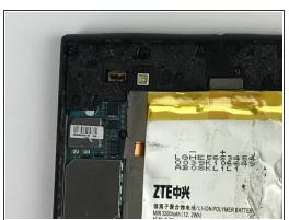
Pull up the piece that is connected to the motherboard. You can pull it using your nails.
