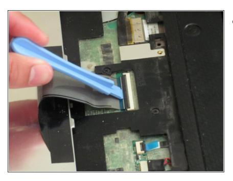
Using a plastic opening tool, flip the ZIF connector up to release the ribbon and the keyboard.
