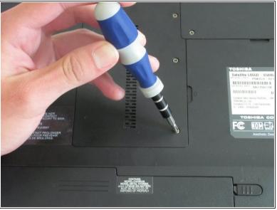
Unscrew the three 4.6 mm screws holding the panel using a #1 size Phillips head screwdriver. The panel is centered on the bottom of the laptop.
