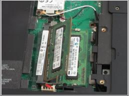
Push the two tabs outwards, away from the RAM. The RAM should spring up.
