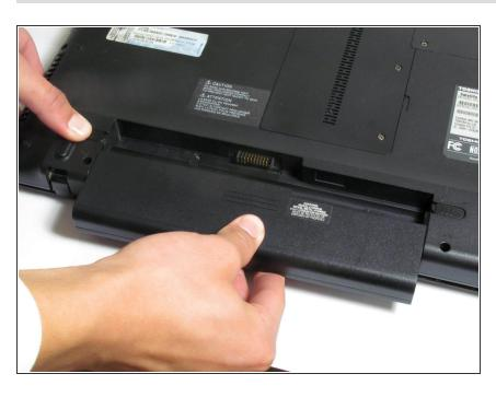
While holding the lock in place, slide the battery out towards you.
