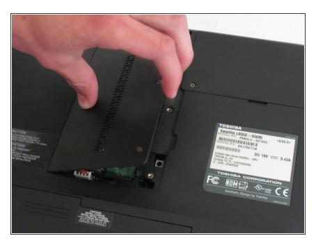
Remove the cover, firmly lifting from the indent. It is recommended that you leave the screws in the panel.
