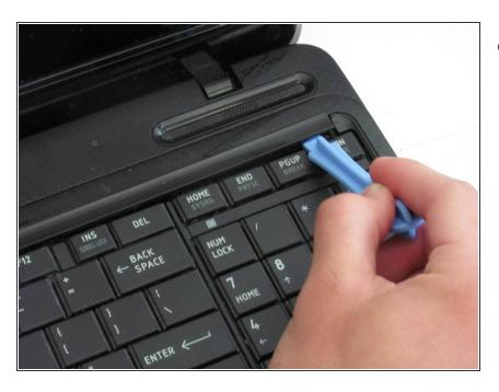
Use a plastic opening tool to pry off the plastic panel above the keyboard.
