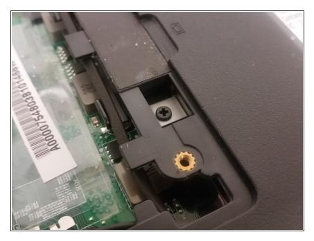
Remove the single screw securing the optical drive, and pull the optical drive out.
