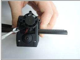
The fan is held loosely in place at the base of the printer head. Use a metal spudger to gently pry it out of the printer head.
