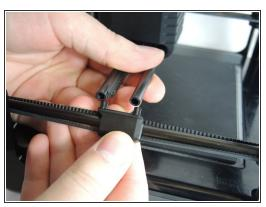
To release the x-rods, pull the x-rods away from the plastic sliders on the y-rods, and flip the slider upwards to release the tracks.
