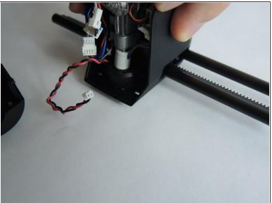
Disconnect the red and black wires at the white connector. They should easily separate.
