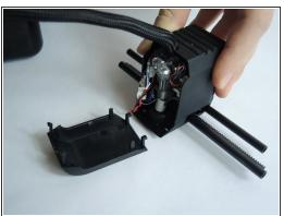
Slide the tracks off the second slider and remove the printer head and x-tracks from the center of the printer. To remove the front cover of the print head, firmly grip the cover and gently pull it off.
