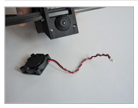
Pull the fan all the way out of the printer head.
