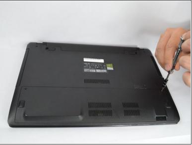
Loosen the two 12 mm screws on the bottom panel of your device using a Phillips size 0 bit.
