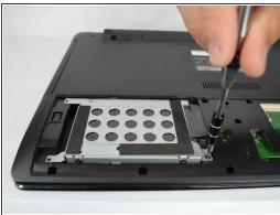
Loosen the three 5 mm screws holding down the hard drive using a Phillips #00 bit.
