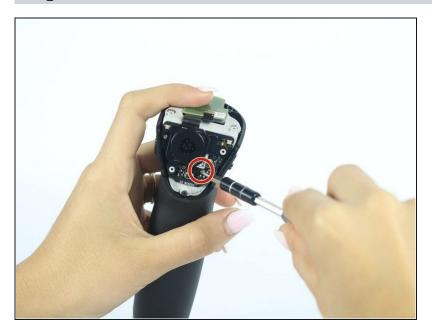
Remove the bottom right screw on the joystick panel with the #00 Phillips screwdriver.
