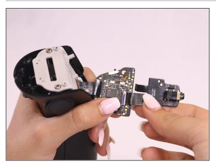
Hold down the larger of the two ribbon cables, and pull on circuit board with a constant and careful down and out motion.
