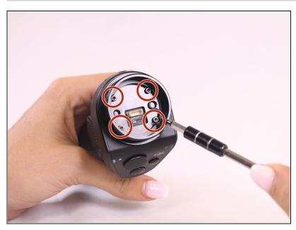
Locate the hex screws found at the top base of the handle, and unscrew using the 1.5mm hex screwdriver.
