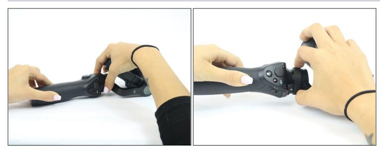
Remove gimbal from base handle by loosening round plate found at the top of the handle.
