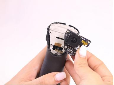
• Gently remove joystick module by pulling it through the circuit board and inserting the new module.
