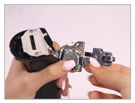
Hold down the larger of the two ribbon cables, and pull on the circuit board with a constant and careful down and out motion.
