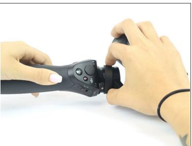
Remove gimbal from base handle by loosening round plate found at the top of the handle.
