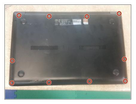
Remove the ten Torx T5 screws securing the bottom cover to the rest of the laptop.
