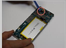
Disconnect all four of the shown electrical connectors by gently prying up with the plastic opening tool.
