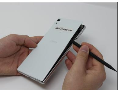
Carefully remove the back panel of the phone with a plastic spudger, or other flat and thin wedge tool. Work your way around the perimeter of the case, loosening and prying gently, until there is sufficient distance between the panel and phone.
