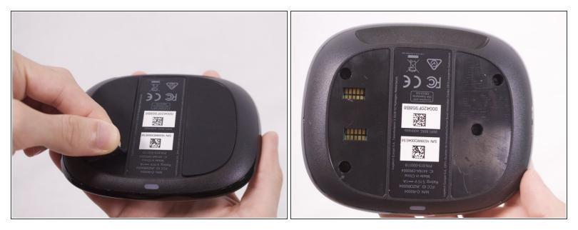
• Remove the non-slip rubber pads on the bottom of the Harmony Hub.
