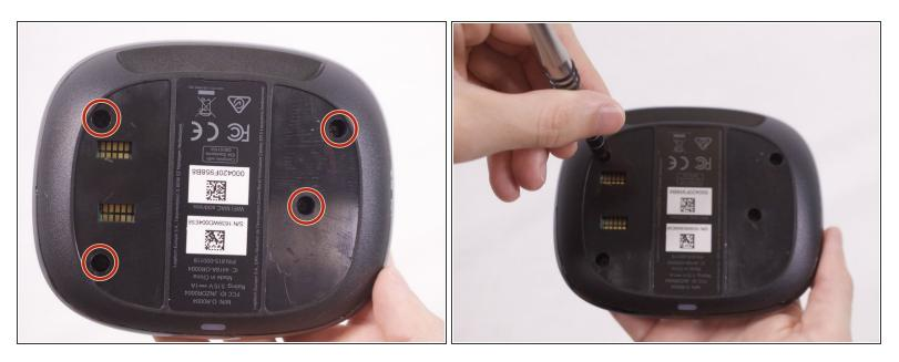
Unscrew the four 6.0 mm Phillips #0 screws.
