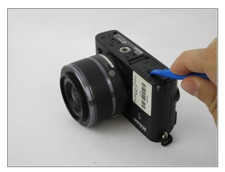
Pull the tab on the bottom of the device
