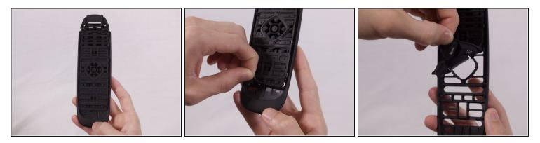
• Lift the button pad up to remove it from the remote.
