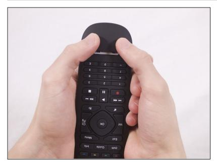
• Push the battery cover upward.
