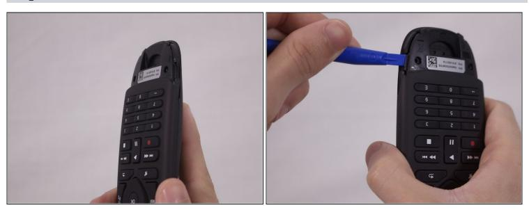
• Use the plastic opening tool to pry open the back cover of the remote.
