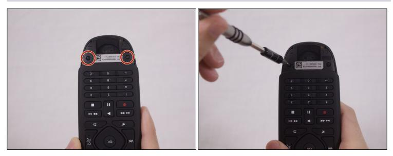
• Remove the two 5.0 mm Phillips #0 screws.
