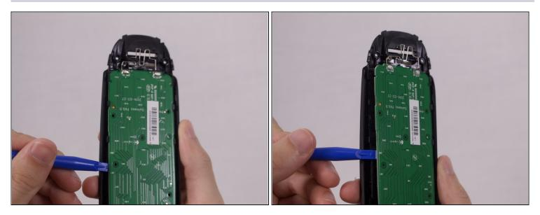
• Use the plastic opening tool to remove the motherboard.
