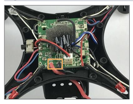
Carefully remove faulty battery wiring from the drone
