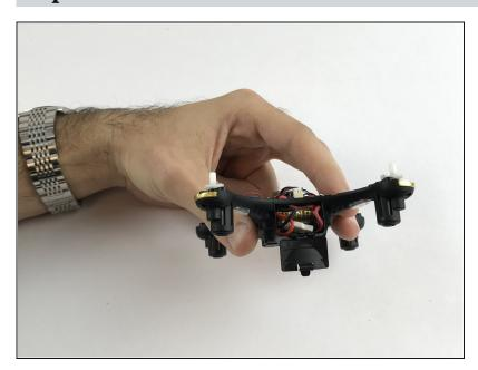
Open the hatch and carefully pull out the battery to expose the cable connection
