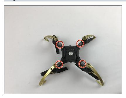
• Reattach the battery and test for power by turning on the drone and look for the 4 LEDs turn on.
