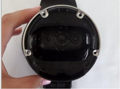
Remove the 6 screws from the seal with a Phillips #1 screwdriver.
