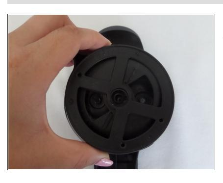
Twist the black lid on top clockwise until it is completely detached.
