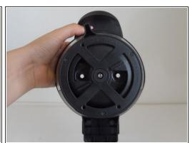
Hold the head in the same position and lift it forward until the Ninja is facing upward toward the ceiling.
