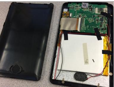
Carefully pry the back cover off of the tablet. It may take quite awhile to get the cover off, be careful to not damage any of the clips.
