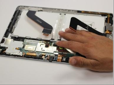
• Remove the battery connecter by gently pulling up with your finger.
