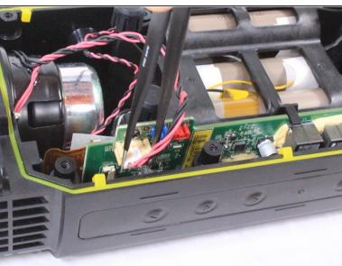
Carefully untangle and remove the white bundled cable connectors from the motherboard.
