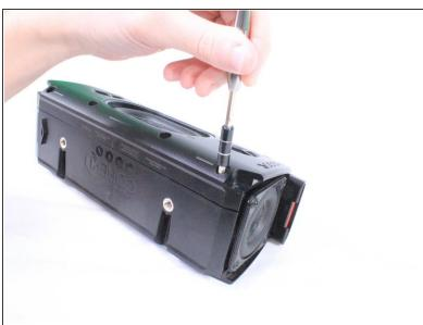
Use a #2.0 Hex screwdriver to unscrew the 8 screws shown in the image.
