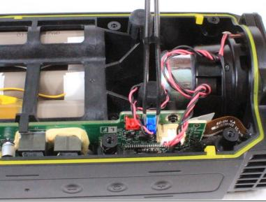
Untangle any blue bundled cable connectors and gently remove them from the motherboard using a pair of tweezers.
