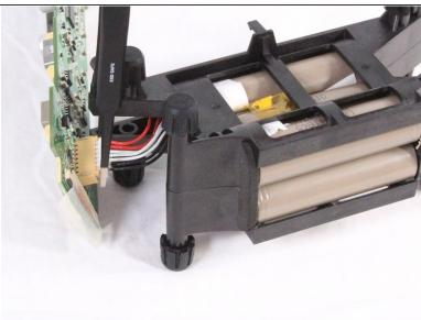
Using tweezers or your hand, carefully disconnect the bundled cables connecting the battery to the motherboard.
