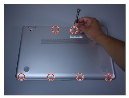
Remove the six 5 mm Torx screws using a T5 Torx Screwdriver.
