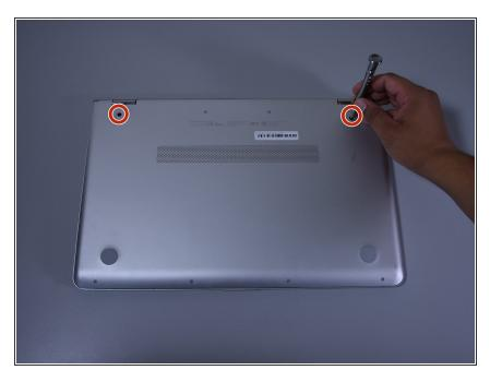
Remove the two 8 mm Phillips Head screws that were under the grip pads using a Phillip's Head 1 Screwdriver.
