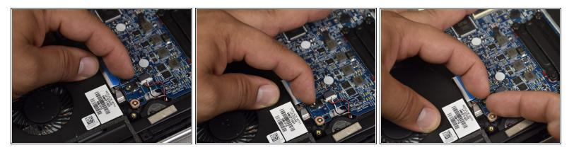
• Disconnect the port with the red yellow and blue wires by dislodging the wires with your fingers.
