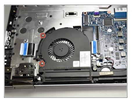
Remove the two 4.5mm Phillips #1 screws.
