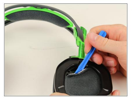
Squeeze the plastic opening tool between the black plastic and foam pad on non mic side and then pry upwards to remove the felt pads covering the speaker.
