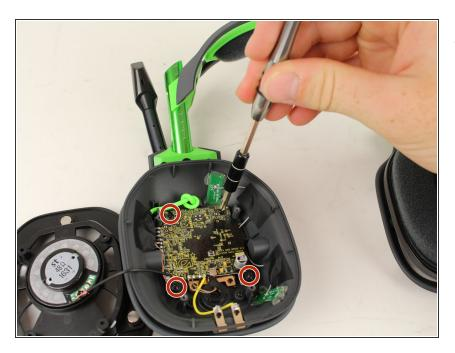
Remove the four 6mm Phillips 1 screws.
