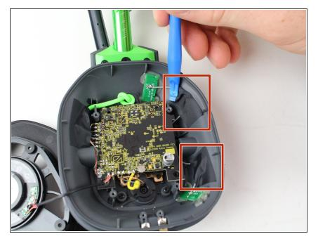
Use the plastic opening tool to pry off the black tape covering the gray wires
