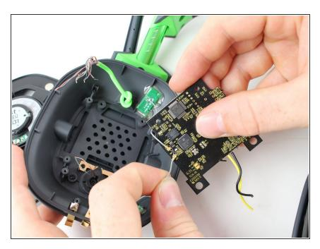
• Lift the motherboard out of the headset and gently disconnect the gray wires from the motherboard.
