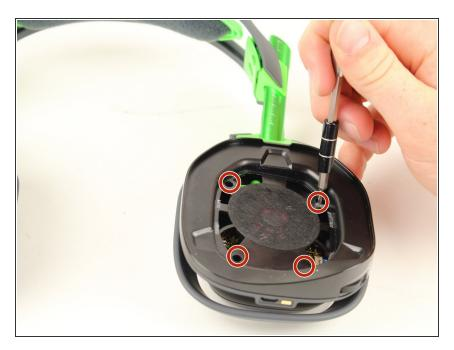
Remove the four 6mm Phillips 1 screws.
